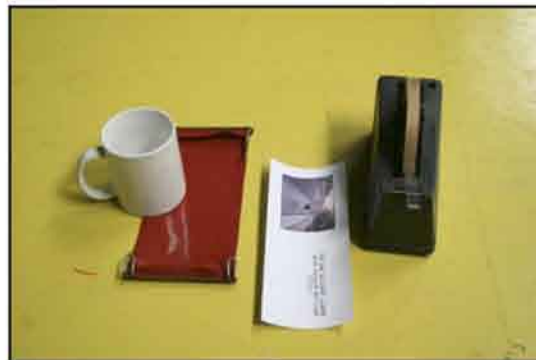
Supplies needed: UltraWrap, sublimation transfer, heat tape, and mug.
